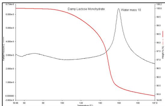
Figure 7 TG-MS Plot of Lactose Monohydrate Dehydration after atmospheric exposure for 24 hrs
