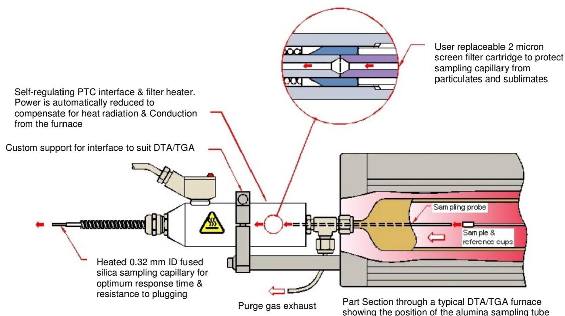
Figure 1 Example of a Hiden TGA-MS Interface
