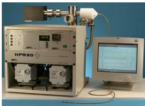
Figure 2 HPR-20 QIC Mass Spectrometer
