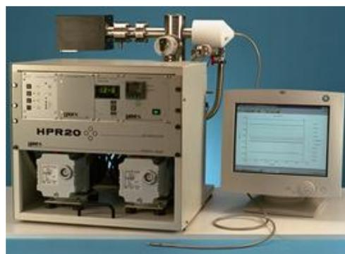
Figure 2 HPR-20 Mass Spectrometer
