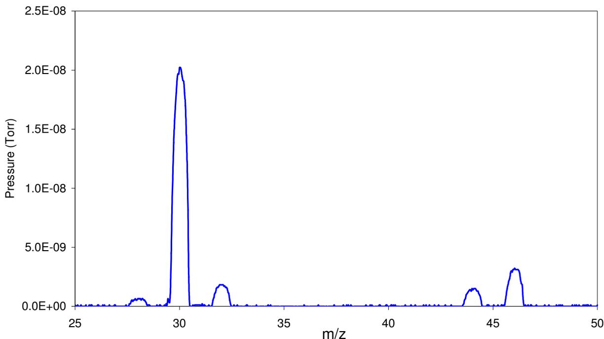
**Figure 1: Profile scan for 10000ppm NO<sub>2</sub>.**
