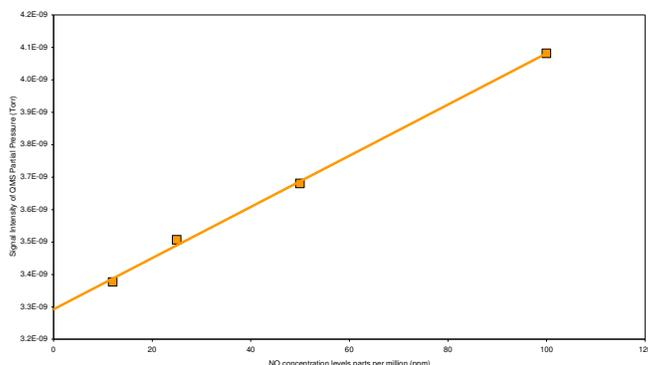
**Figure 3: Relationship between partial pressure for m/z 30 and NO concentration (Note: The background at m/z 30 due to NO<sub>2</sub> has been subtracted).**
