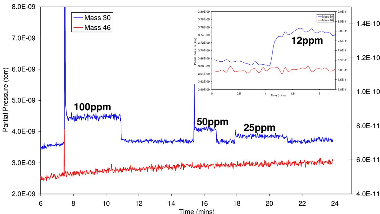
**Figure 2: Detection Limit of NO in 1000ppm NO<sub>2</sub> (Inset: Expansion of detection of 12ppm NO in 1000ppm NO<sub>2</sub>). Primary Axis represents Partial Pressure at m/z 30, Secondary Axis represents Partial Pressure at m/z 46.**
