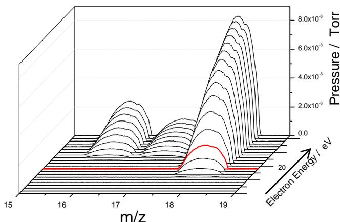
Figure 1 A: m/z vs Electron energy-H<sub>2</sub>O/Air
