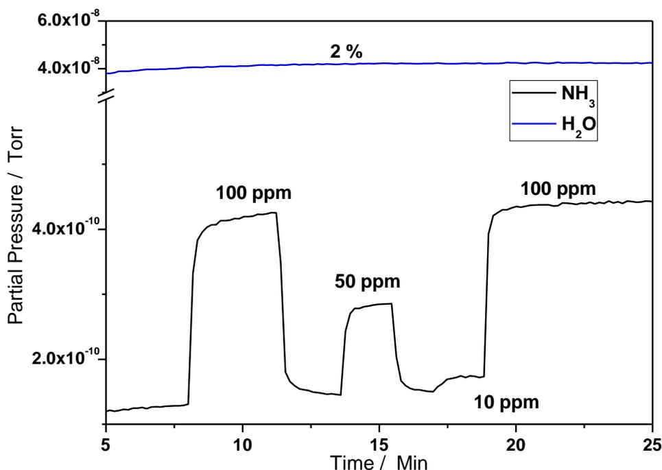
Figure 3: Detection limits of NH<sub>3</sub> in 2% H<sub>2</sub>O
