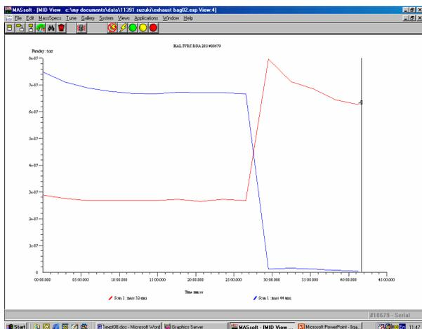
Figure 3: MID mode of Oxygen / Carbon Dioxide peaks.
