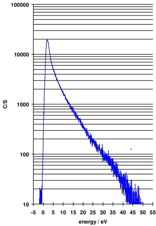
Figure 2 Cu Ion Energy Distribution (logarithmic plot)
