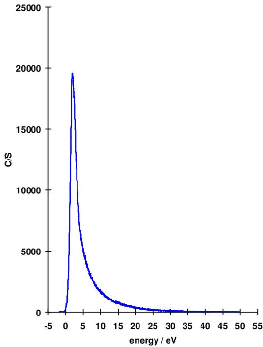
Figure 1 Cu Ion Energy Distribution
