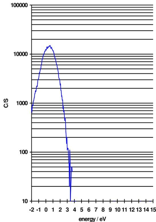
Figure 6  $m/e=26$  Atom Energy Distribution (Plasma On)
