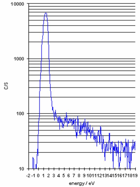
Figure 10 Cu Atom Energy Distribution
