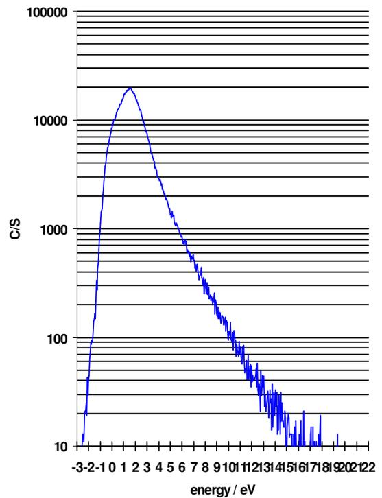
Figure 8 Cu Ion Energy Distribution
