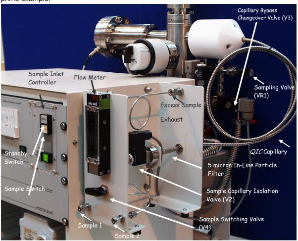
Figure 1: QIC Dual Stream Capillary Connection Kit mounted on HPR-20 QIC system.
