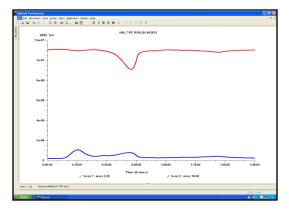
Figure 4 TPR of Plasma modified Ni/MgO Catalyst
