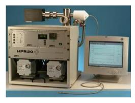
Figure 2 HPR-20 Mass Spectrometer
