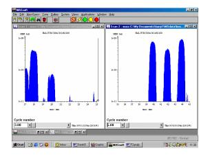
Figure 4. Kr before (a) and after (b) F<sub>2</sub> analyses
