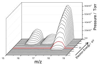
Figure 1 A: m/z vs Electron energy-H<sub>2</sub>O/Air
