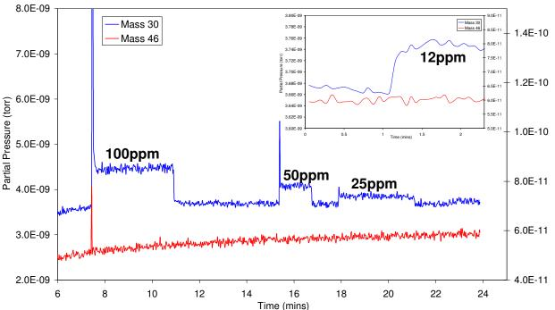
Figure 2: Detection Limit of NO in 1000ppm NO<sub>2</sub> (Inset: Expansion of detection of 12ppm NO in 1000ppm NO<sub>2</sub>). Primary Axis represents Partial Pressure at m/z 30, Secondary Axis represents Partial Pressure at m/z 46.
