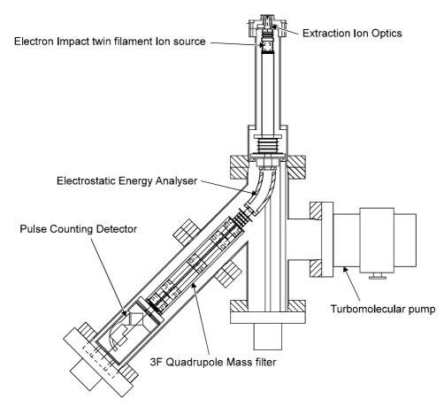
**Figure 1 EQP Mass Spectrometer**
