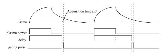
Figure 4 Pulsed plasma afterglow monitoring
