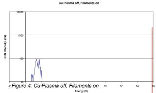
Figure 4 shows that these ions, as expected, have an energy range of about 2eV, centred at approximately The difference between the 1.5eV. distributions of Figure 3 and 4 is consistent with the interpretation of the high energy range of Figure 3 as being due to the ejection of energetic copper atoms from the magnetron's cathode.
