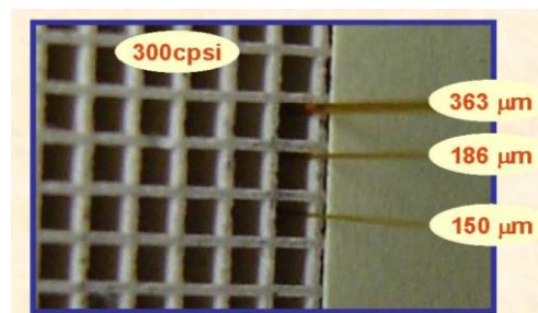
Figure 3. Channelized monolithic catalyst showing SpaciMS capillary sampling probes of various sizes.
