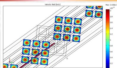
Gas distribution and velocity inside the monolith channels.
