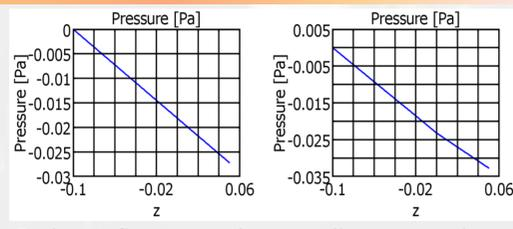
Probes influence in the overall pressure drop of the gas inside the channel. Without probe (left) and with a 250 μm probe (right).
